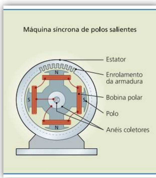
**Figura 22 - Motor Corrente Alternada.**
