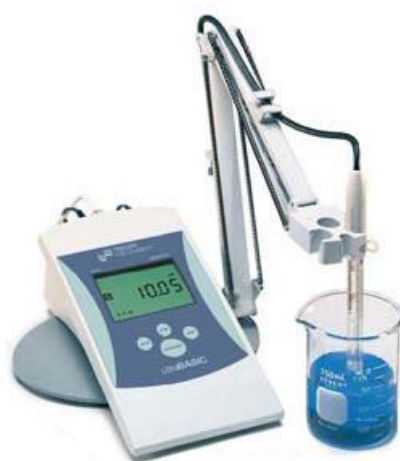
Figura 29 – pHmetro Denver Instrument UltraBasic Benchtop. Fonte: Fisher Scientific (2014).
