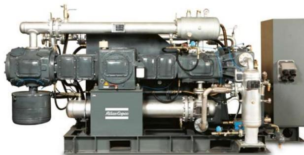
**Figura 30 - Compressor Atlas Copco P65-60**
