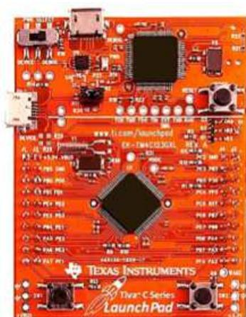
Figura 13 - Kit Microcontrolador *LaunchPad* Tiva C Series TM4C123G (TEXAS INSTRUMENTS, 2013).
