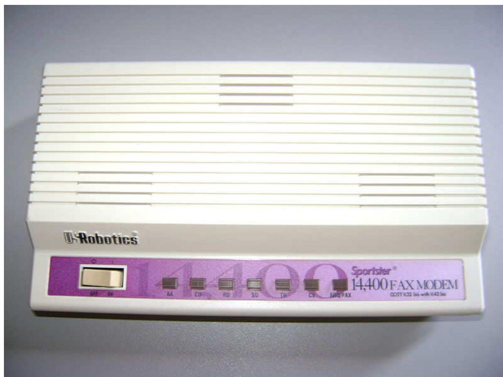
**Figura 3 - Modem externo *US Robotics*.**
