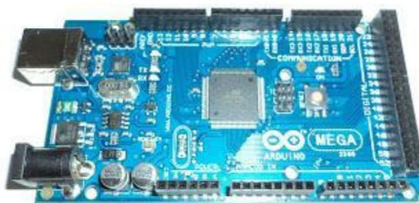
**Figura 36 – Arduino Mega2560**
