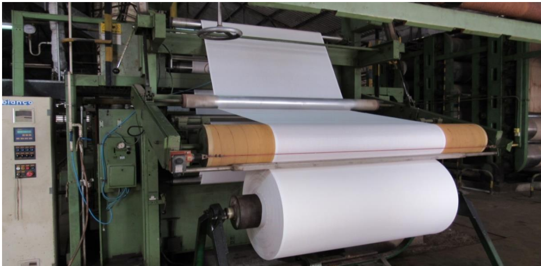
Figure 7 - Stretching before printing Source: Elaborated by the author (2019)
