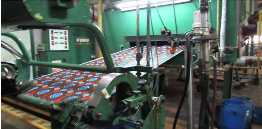
Figure 10 - The second application of dye Source: Elaborated by the author (2019)
