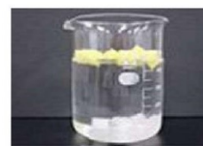
Water floating polyurethane sponge (yellow) and water sinkable AQUAPOROUSGEL "CC-10B" (white)
