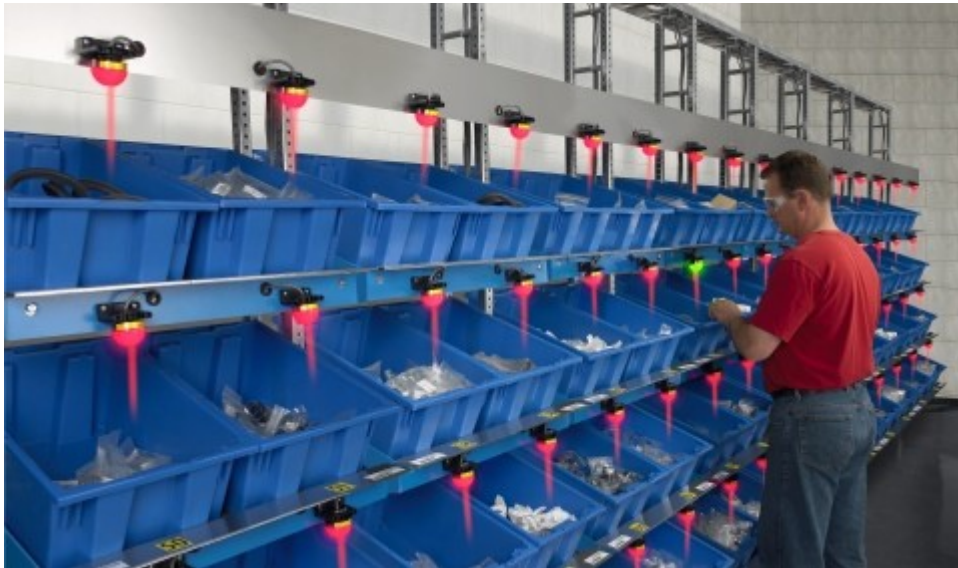
Figura 6 – Processo “Pick to light”
