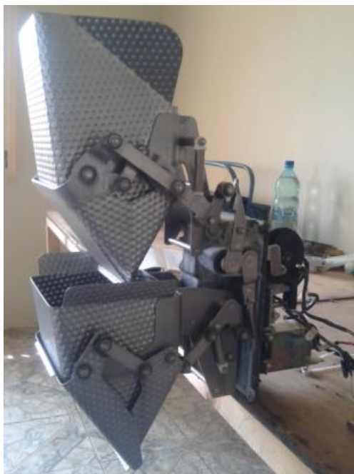
Figura 22: Cabeçote Multihead Weigher.
