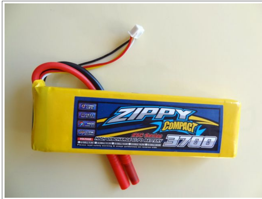
Figura 27 – Bateria Zippy Compact LiPo 3S 25C 3700mAh.
