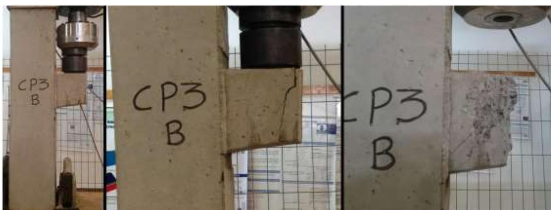
**Figura 51 – Ruptura CP<sub>norma3</sub>**
