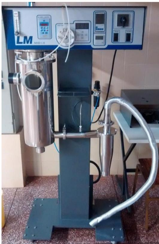
**Figura 6-** Mini Spray Dryer, MSD 1.0 LABMAQ.
